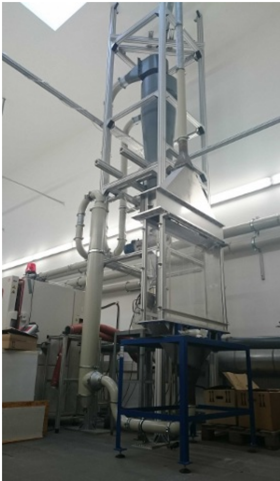
Laboratory spray dryer for the investigation of the interaction (collisions) of dry droplets by using two interacting flat jet nozzles.
